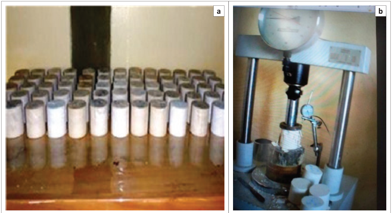
FIGURE 7: (a) Cylindrical plaster of Paris (POP) models for compressive testing; (b) A Germany Universal Testing machine (UTM), or materials test frame, is used to test the tensile strength and compressive strength of materials.
