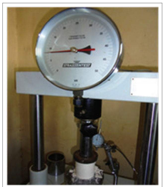
FIGURE 9: A Germany Universal Testing machine (UTM), or materials test frame, is used to test the tensile strength and compressive strength of materials.
