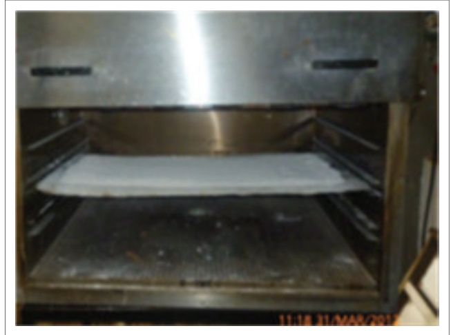
FIGURE 6: Heat oven for heating polypropylene plates used for molding different parts of assistive mobility devices.
