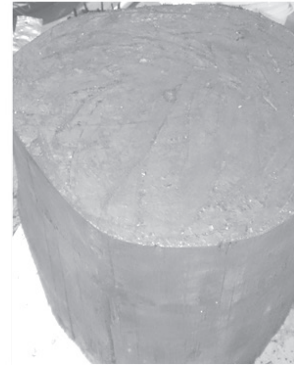
Fig. 4. Wood samples for capacitance measurement
