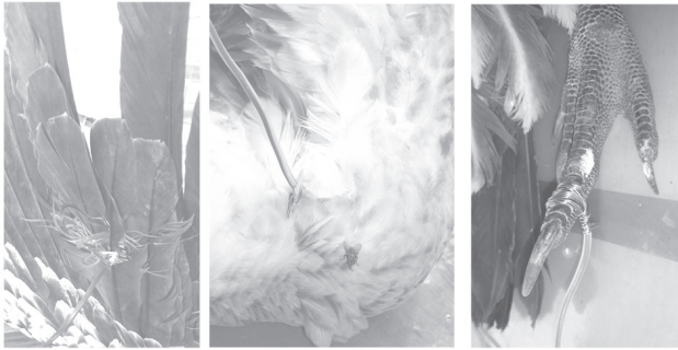
Fig. 7. Electrode connections to wing feathers (left), wing shoulder (centre) and foot (right)
