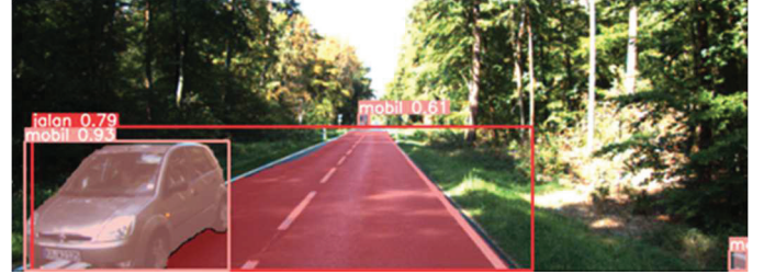
Fig. 8. Sample of road and car detection using the KITTI dataset.
