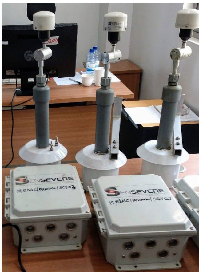
Figure S1: The RAMPs and the external Met-One NPMs in the lab (left) and a unit deployed in Kigali, Rwanda (right).
