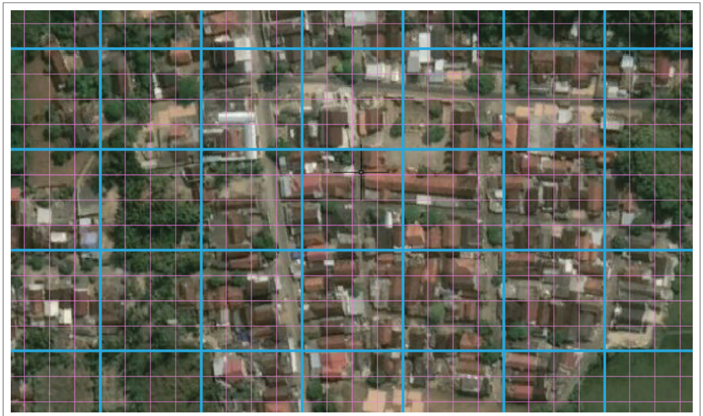
FIGURE 8: The difference in size is 50 \times 50 and 12.5 \times 12.5 in the grid cell system.
