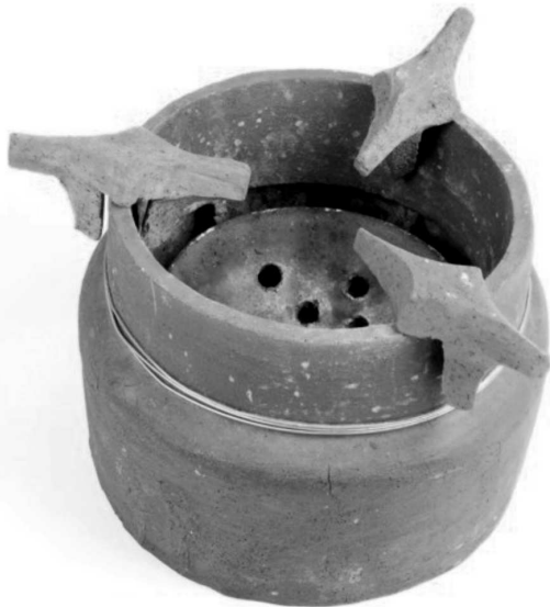
Figure 2: Maputo Ceramic Charcoal Stove, 2008 (showing charcoal burn area and air gap surrounding it) (Photograph: A. Campbell)
