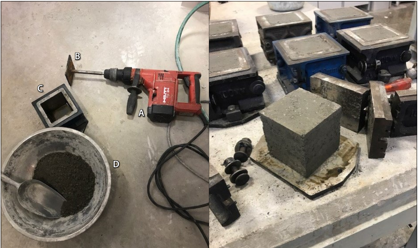
Figure 3 The left-hand image shows (A) the percussion drill, (B) the modified tool bit, (C) a steel cube mould and (D) the zero-slump concrete used (in a funnel); the right-hand image shows a de-moulded sample for the green-state strength test
