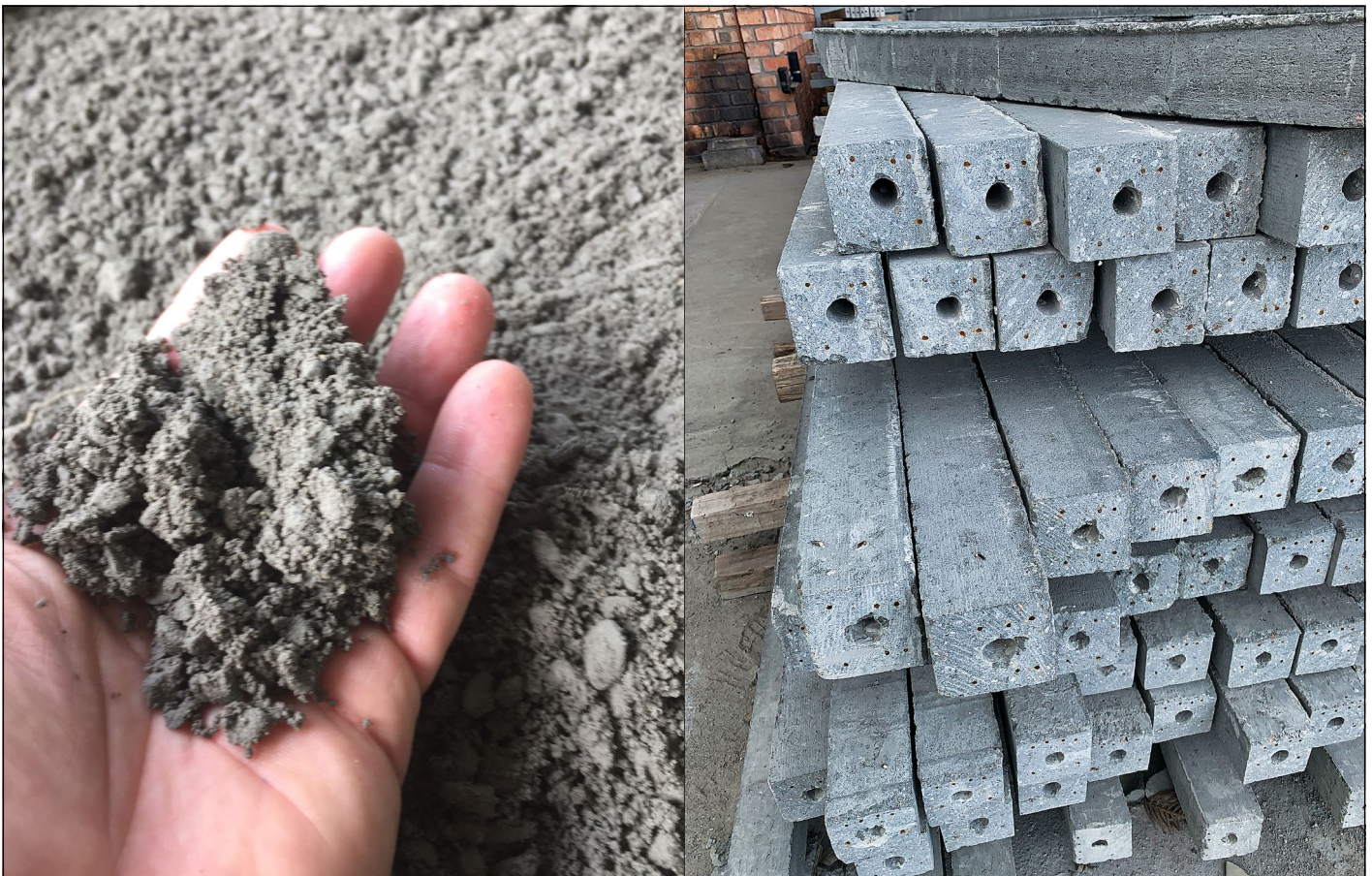
Figure 2 The left-hand image shows the loose texture of the zero-slump concrete that was investigated in a particular precast plant, while the right-hand image shows precast lintels made with this mix
