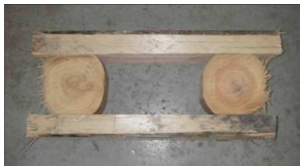
Figure 2—55 x 27 x 11 cm Timrite Lexus: stope support pack
