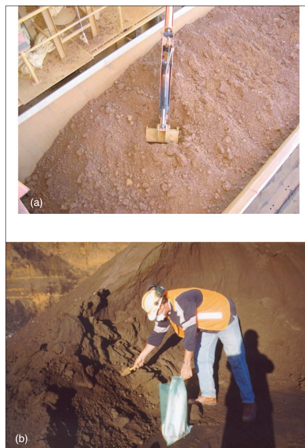
Figure 17—Sampling from (a) the top of railway wagons and (b) the side of stockpiles will not provide representative samples
