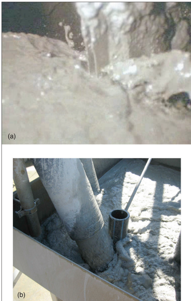
Figure 13—Examples of (a) a full cross-stream slurry sampler and (b) manual sampling of a slurry stream using a ladle that is too small for the stream being sampled
