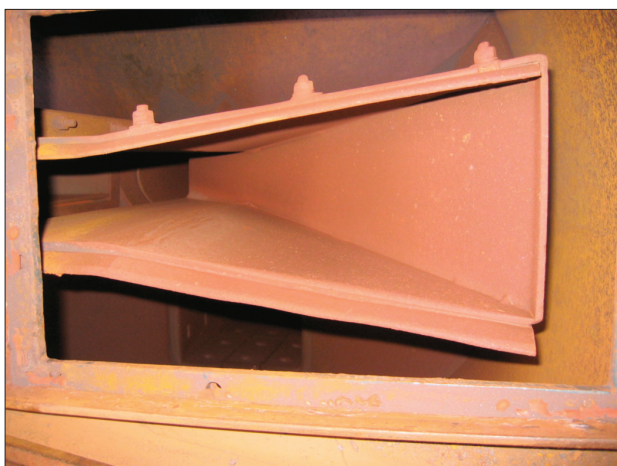
Figure 1—Correctly designed rotating Vezin cutter with radial cutter lips
