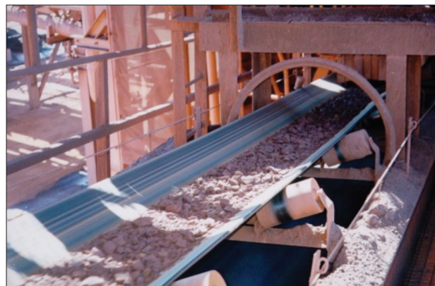
Figure 3—Moisture loss from an open slow moving conveyor transferring primary increments from the primary cutter to the secondary cutter
