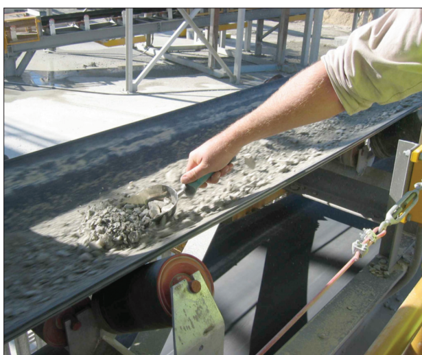
Figure 10—Manual sampling from the top of a conveyor belt raises serious safety concerns and in any event does not provide a representative sample
