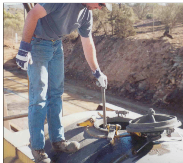
Figure 11—Manual sampling of vessels using a ladle is not recommended due to segregation of the material in the vessel
