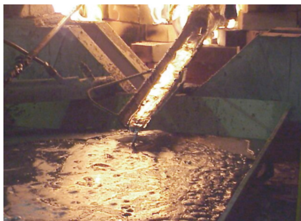
Figure 5—Online magnesium tapping—Run 5
