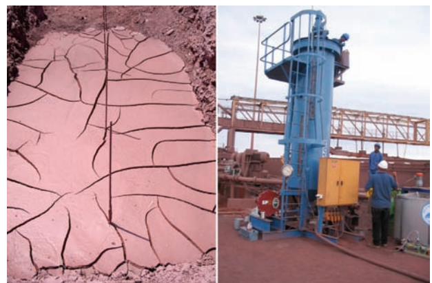
Figure 4—Feasibility paste pilot plant and flume test work conducted at Beeshoek Mine
