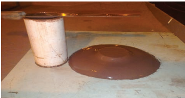
Figure 15—A slump cone test on a sample taken from the proving loop
