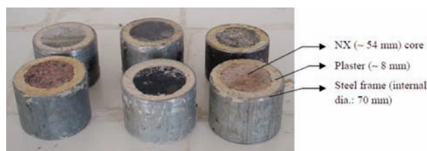
Figure 1—Cemented samples in the circular steel frames
