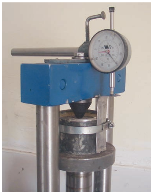
Figure 2—Indentation testing using point load apparatus
