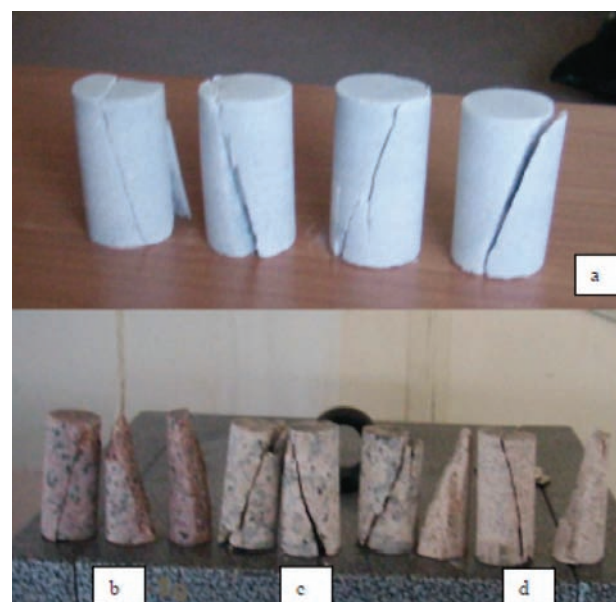
Figure 4—Some samples failed in the uniaxial compression test: a) Milas/Mugla marble, b) unknown granite (King Rosa), c) Kaman/Kirsehir granite (Kaman Rosa), d) Porrino/Spain (Pink Porrino)
