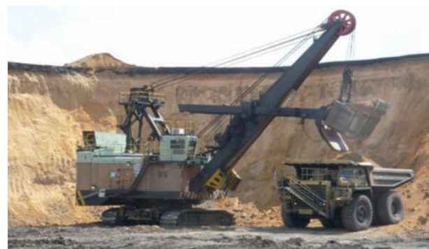
Figure 3—Current single-sided loading method
