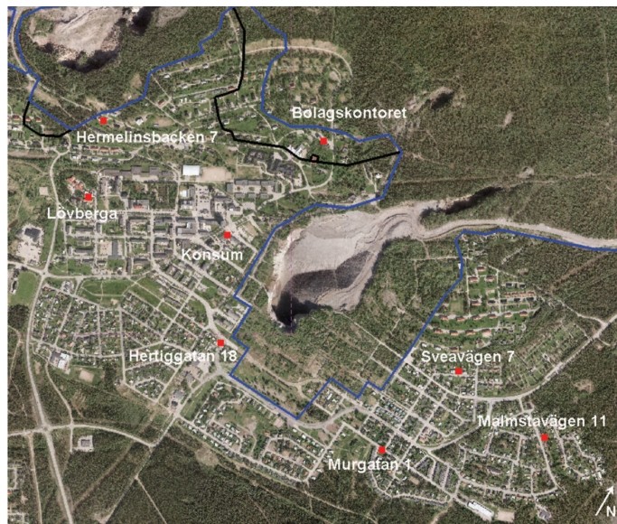
Figure 6—Vibration monitoring points in MalMBERGET town. Blue line is the industrial fence, and black line is recent fence advancement
