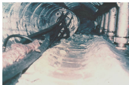
Figure 2—Stope coring of gold reef
