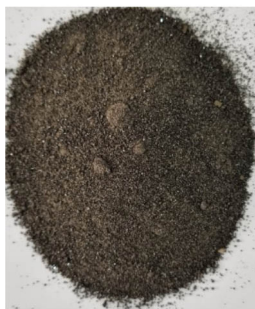
Figure 14—Material gathered from cutting UG2
