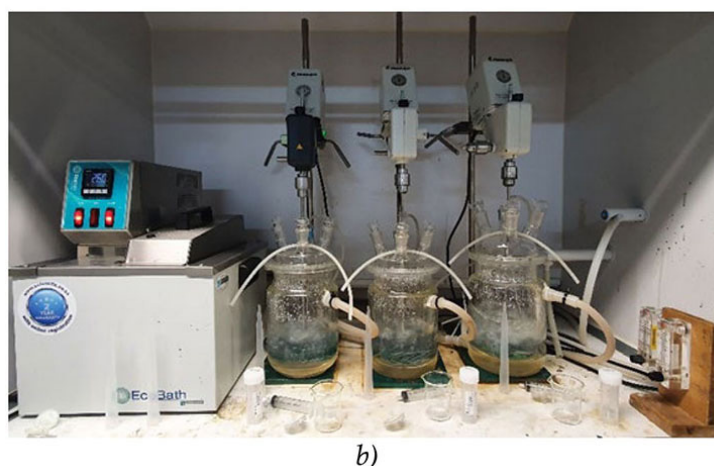
Figure 2—a) Schematic of the batch stirred tank reactor (BSTR); b) Reactor set-up with a heating water bath, 3 BSTRs and air supply
