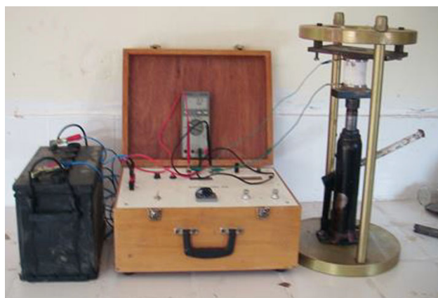
Figure 1—The experimental set-up used for measuring electrical resistivity
