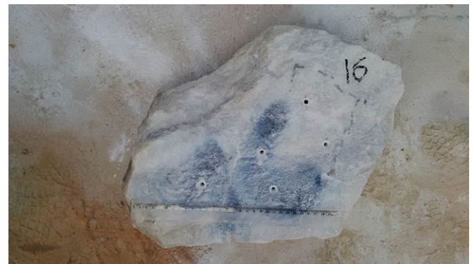
Figure 3—A block with drilling set out to simulate distributed charges for PF_{th} = 0.3 \text{ kg/m}^3
