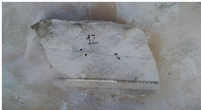
Figure 2—A block with drilling set out to simulate concentrated charges for PF_{th} = 0.3 \text{ kg/m}^3
