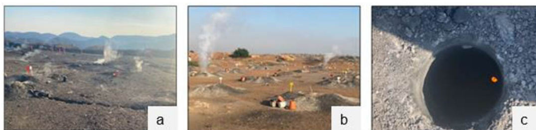
Figure 2—(a, b) Venting holes and (c) a fire in a hot hole at a mine that has hot-hole challenges
