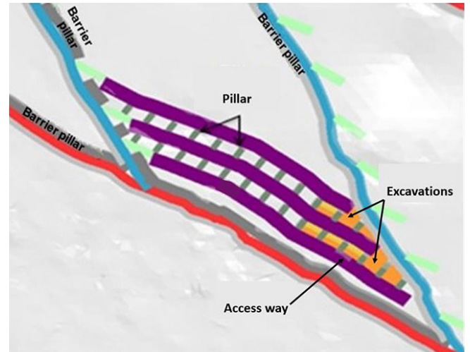
Figure 4—Positions of main support structures and initial stages of development (plan view)
