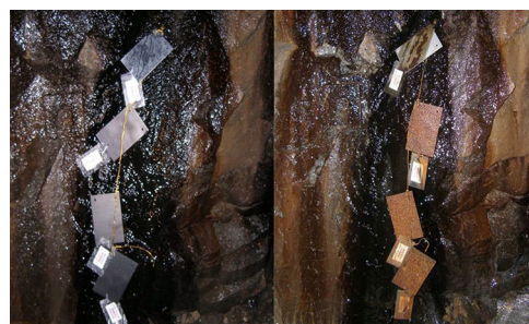
Figure 2—Corrosion coupons in a wet environment: (a) on installation, (b) 12 months, Dorion et al. (2010)
