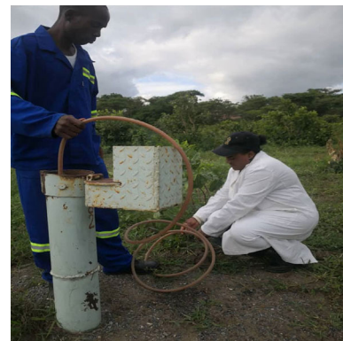
Figure 7—Water sample being collected from one of the monitoring boreholes
