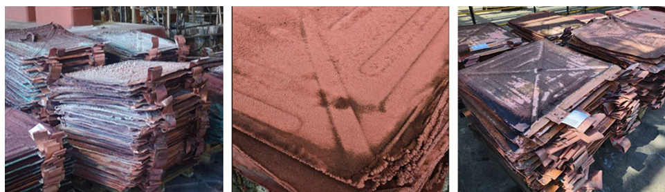
Figure 9—Poor-quality mossy copper, with excessive nodulation, and the effects of high selenium and tellurium impurities
