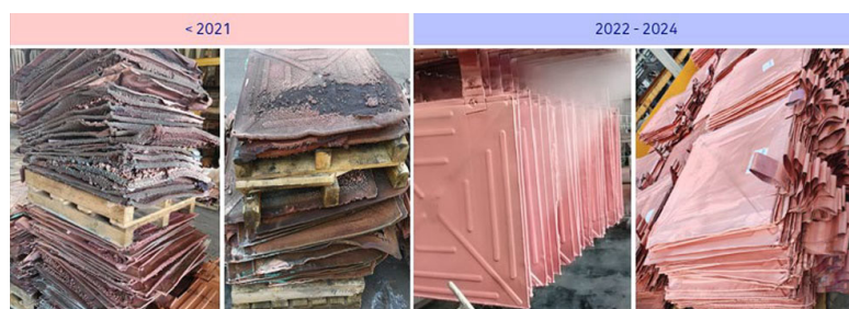
Figure 12—Comparison of poor-quality (mossy copper) production frequently achieved prior to 2021 with present, high-quality production
