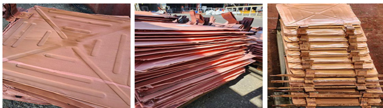
Figure 11—Good quality, smooth copper cathode with minimal nodulation, defects, and dendrite growth
