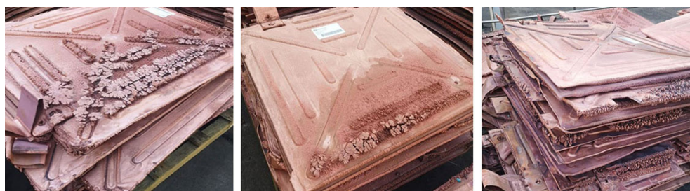
Figure 10—Effects of short circuits on copper cathode production owing to inadequate fault checking and rectification, leading to excessive nodulation and dendrite growth
