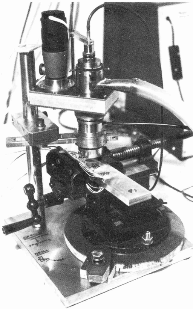
Figure 5 Photograph of the drilling unit. Note, from the top, the drilling unit can be seen held in the guide bush with the air-alumina and vacuum hoses connected to it. Beneath it is a calibration specimen which is held in a rotational 2-D cross vice.
