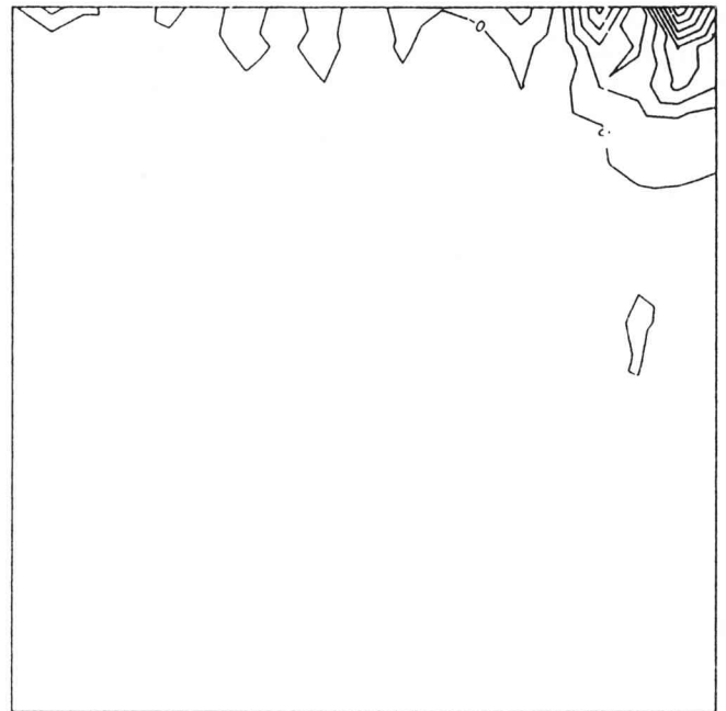
Figure 7 Contours of the absolute U-velocity component integrated source terms for central difference discretization — 41 \times 41 nodes
