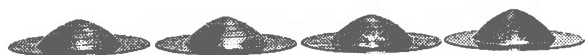
Figure 13 Pictures of deformed copper disks. Thickness 0.9 mm. From left to right: 16.03, 17.22, 17.5, 19.0 mm midpoint deflection
