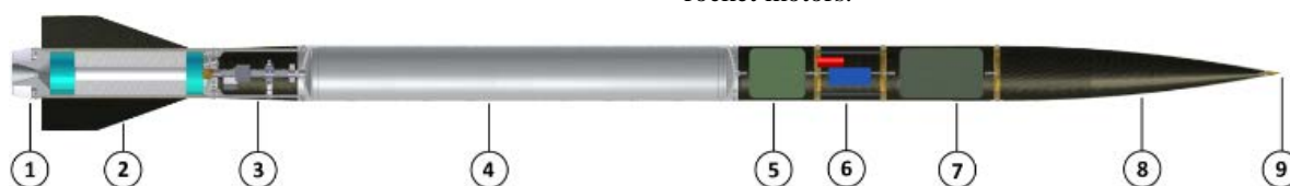
1) Boat-tail, 2) PV-1 Flight Motor, 3) Oxidiser Feed System, 4) Oxidiser Tank, 5) Drogue Parachute Bay, 6) Flight Computer Bay, 7) Main Parachute Bay, 8) Nose-Payload Compartment, 9) Aluminium Nose Tip
