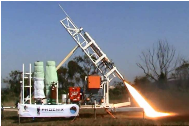
Figure 10 Successful hot-fire test of PV-1 motor, August 2013.
