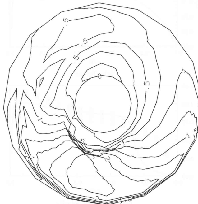
Figure 10 – Thrust distribution for fan with circumferentially distorted inflow
