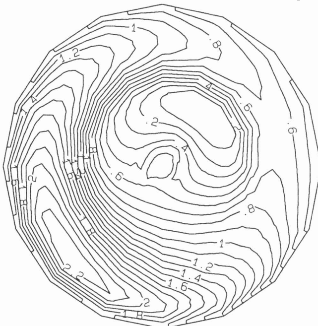
Figure 12 – Predicted u/U contours for fan with circumferentially distorted inflow
