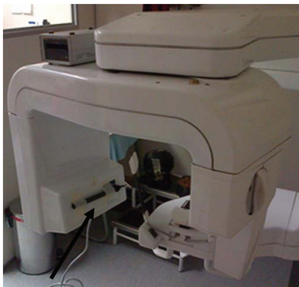
Figure 1: CT pencil ionisation chamber across the width of the receiving slit of the secondary collimator.
