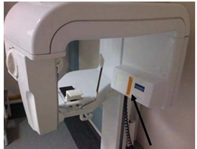
Figure 2: A piece of film on the receiving slit of the secondary collimator.
