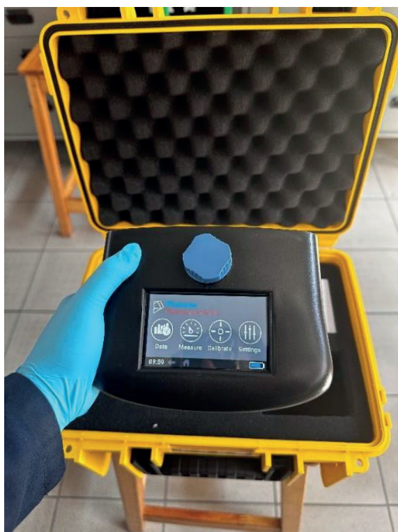
Figure 2: The portable, handheld UV254 Go! analyser.
